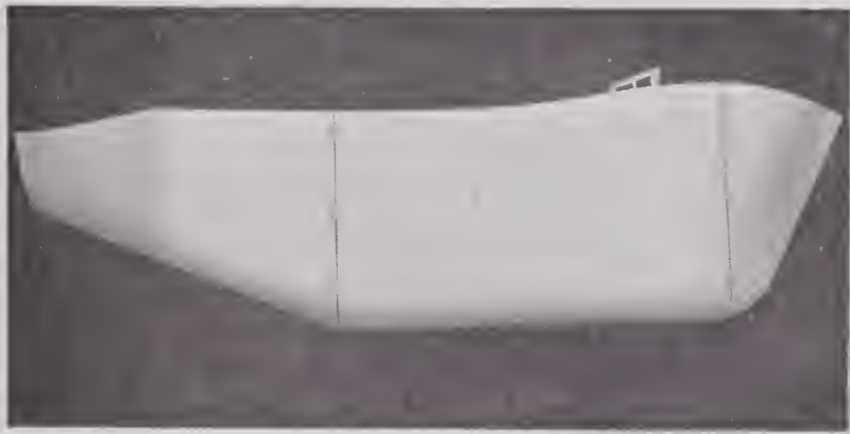
FIGURE 40. New fairing developed for dropping T-15 Weasel by parachute.
